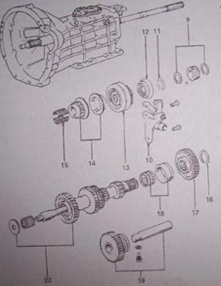
10.10 K50 transmission countershaft, 5th gear and reverse idler gear and associated components
