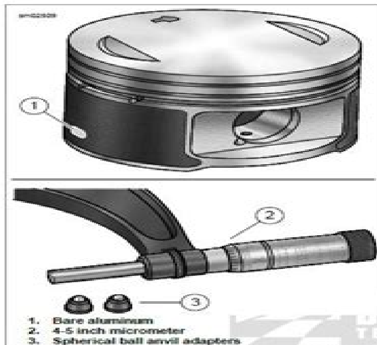
Figure 3-64. Measuring Running Clearance of Piston
