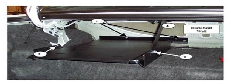
Step 1. Align forward radio shelf bracket with existing holes in front of trunk wall. Use 2 (two) 1/4" x 1" hex head cap screws, 2 (two) 1/4" flat washers and 2 (two) 1/4" flange nuts. Don't fully tighten bracket yet.
