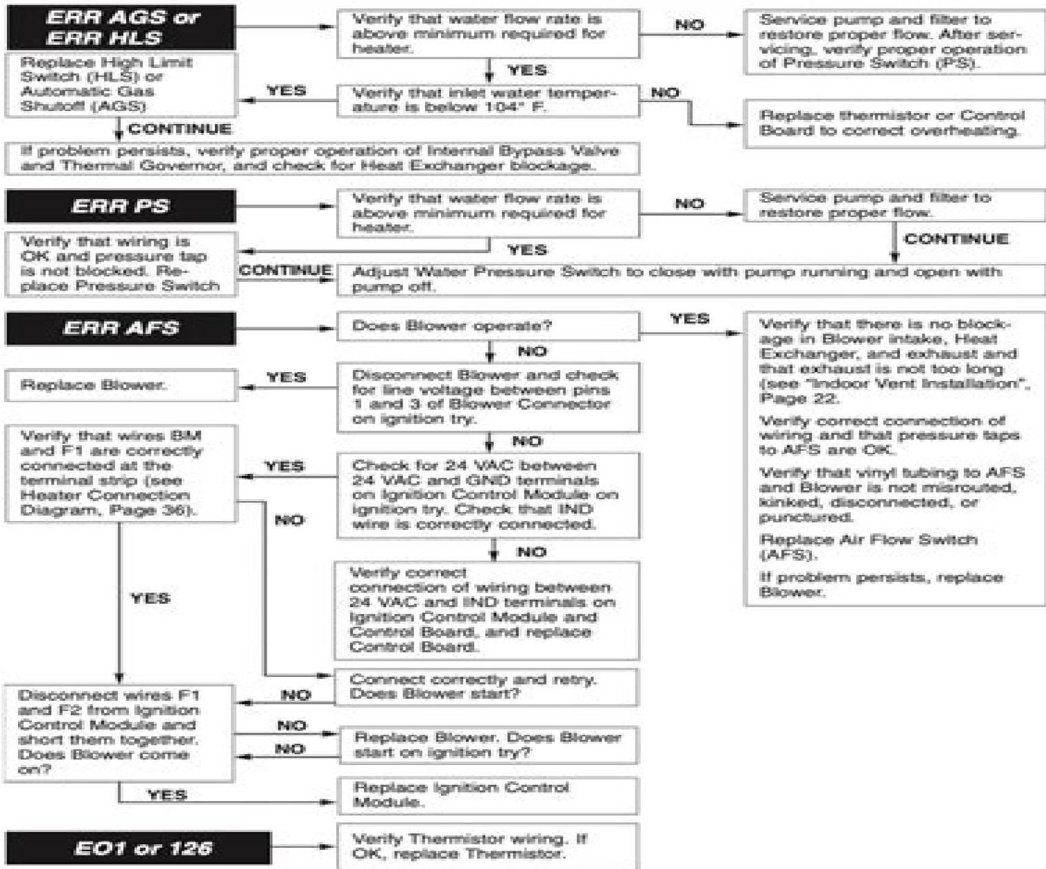
**CAUTION** Do not jumper a safety switch to remedy a failed switch.
