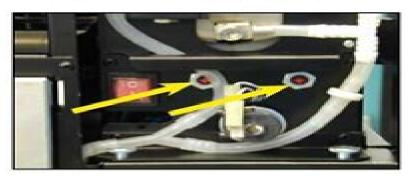
Reset the limit switches by pressing the red knobs until a \_click\* is heard.
