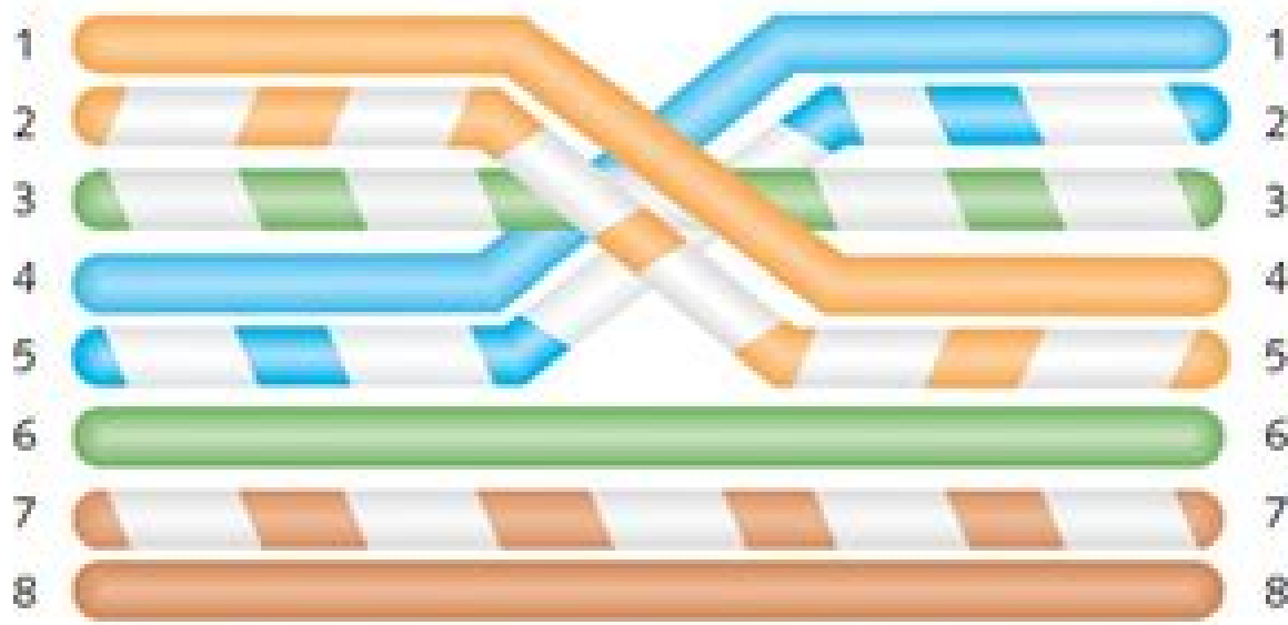
Figure 7-14 T1 crossover cable terminations Courtesy Course Technology/Cengage Learning
