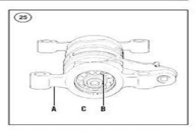
Remove the four dowel pins from the transmission case.
