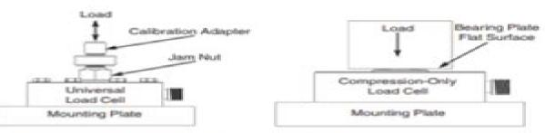
Installation on flat plate per Table 1 or 2 on Page 2 and perpendicular to load axis within 1 degree. Flexure mounting screws to be tightened to the value shown in Table 3 or 4 on Page 2.
