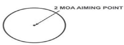
CURRENT VERSION OF M68 CCO's UTILIZE A 2 MINUTE OF ANGLE RETICLE (DOT).
