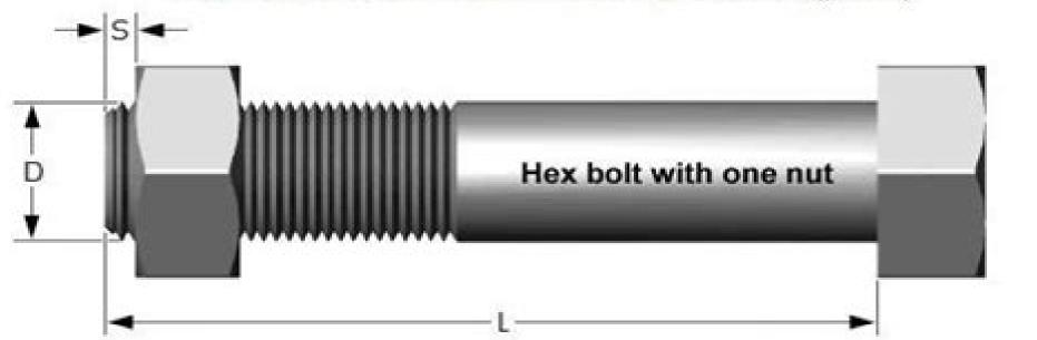
Hex bolts are measured from under the head to the tip of the bolt.
