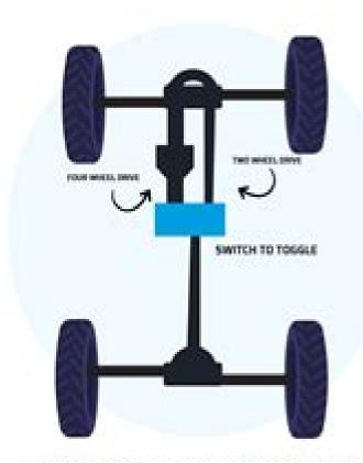
4WD has a selectable switch to choose two-wheel drive mode or four-wheel drive depending on road conditions.
