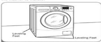
Position the washer in the final location, faking special care to not pinch, strain, or crush the water and drain lines. Place a level across the top of the washer.
