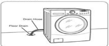
Insert the end of the drain hose into the floor drain. Secure the hose in place to prevent it from moving.
