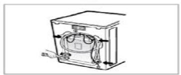
Unscrew the 4 boils with the wrench supplied.
