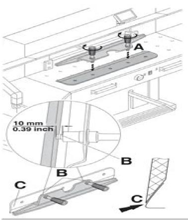
Take the exchange blade carefully out of the blade box and screw it to the blade changing tool (A)
