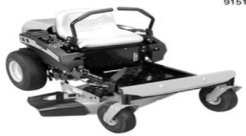
Sasoline containing up to 10% ethanol (E10) or up to 10% MTBE (methyl tertiary butyl ether) is acceptable for use in this machine. The use of any gasoline exceeding 10% ethanol (E10) or 10% MTBE will void the product warranty.
