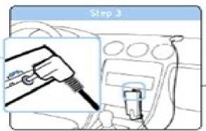
Plag the GPS receiver into the GPS-port and place it in clear view of the sky.
