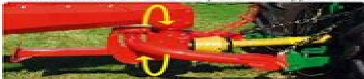
The Gyrodine swivel hitch: 540 or 1000 min -1
