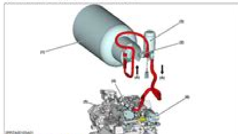
MECHANISM (1) Fuel tank (2) Fuel filter (3) Fuel line (4) Fuel injector (5) Intake manifold (6) Fuel pressure sensor
