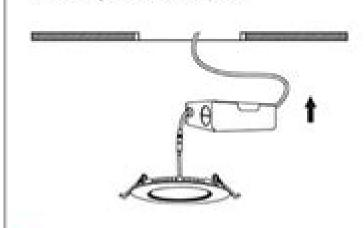
4. Squeeze the snap spring clips and push the light into the ceiling and done!
