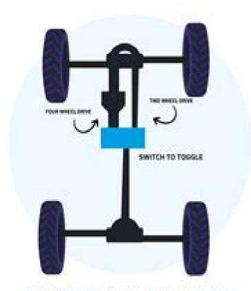
4WD has a selectable switch to choose two-wheel drive mode or four-wheel drive depending on road conditions.
