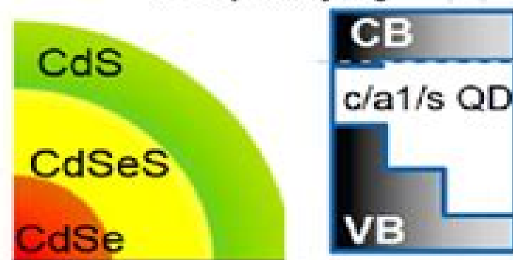
b Core/alloy/shell QD with 1-step alloying
