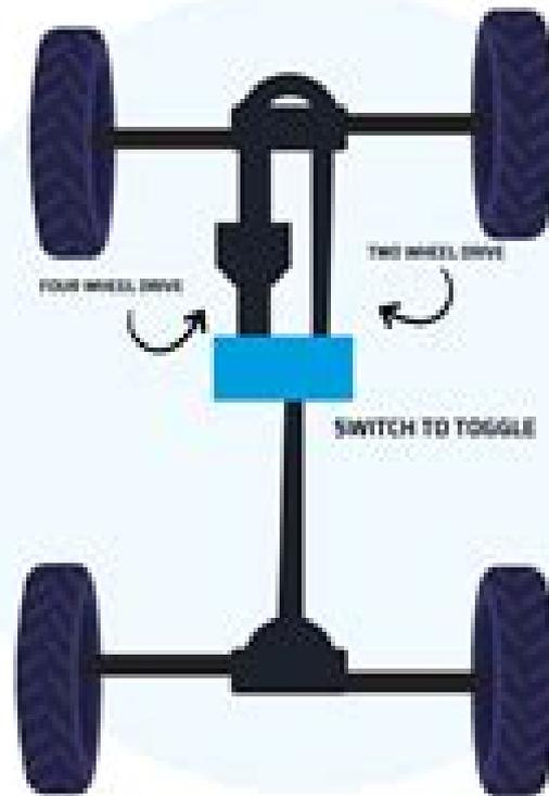
4WD has a selectable switch to choose **two-wheel drive** mode or **four-wheel drive** depending on road conditions.
