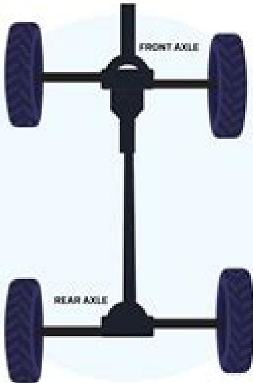
AWD sends power to either the **front axle** or **rear axle** in normal driving conditions. If the vehicle detects a lack of traction it will **engage** to all wheels.
