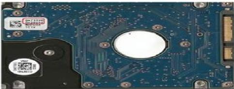
Swapping the printed circuit board (PCB) on Hitachi hard drives requires matching 4 things "EXACTLY" for your best chance of success without having to swap any chips from your old PCB to the new PCB.
