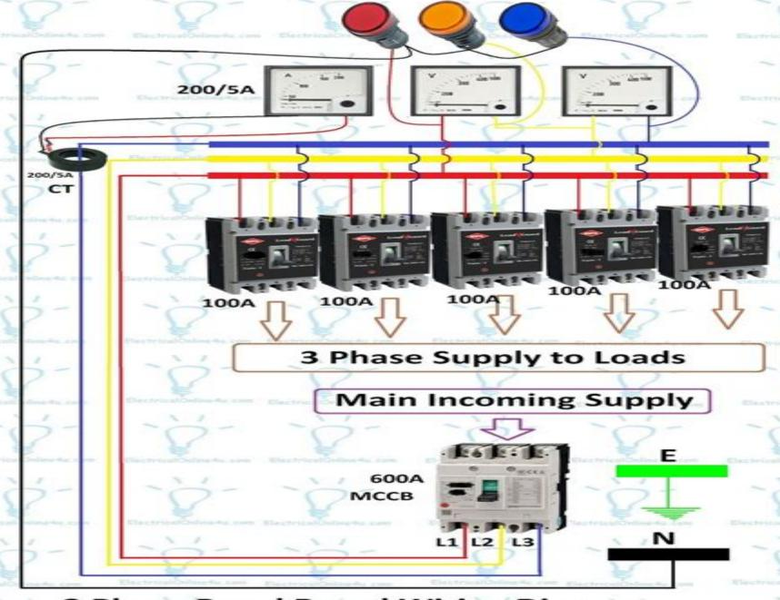
3 Phase Panel Board Wiring Diagram
