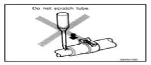
To reinstall the rubber hose securely, make sure that hose insertion length and orientation is correct. (If tube is equipped with hose stopper, insert rubber hose into tube until it butts up against hose stopper.)
