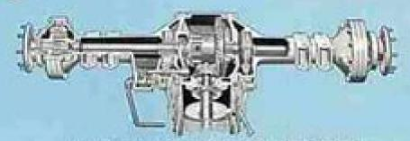
Rougardly count run axis his final reduction through totally exchand out bath spacyclin hab pears giving final drive reduction of 1:10.9. Note also the two implement resourcing poles and differential lock liant polal. Disc brakes acting independently—are scaled against weather, goe double-quick turnersual.
