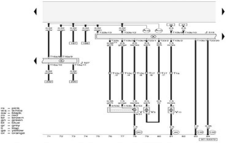
J519 - Vehicle Electrical System Control Module
