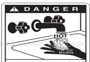
Water temperature over 125° F (52°C) can cause severe burns instantly or death from scalds.
