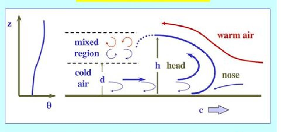
Schematic diagram of a steady gravity current
