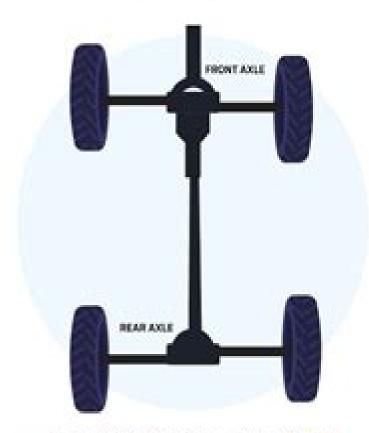
AWD sends power to either the front axle or rear axle in normal driving conditions. If the vehicle detects a lack of traction it will engage to all wheels.
