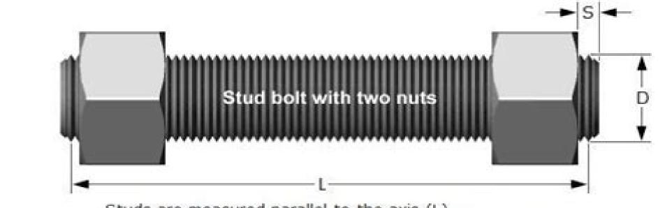
Studs are measured parallel to the axis (L) from the first to the thread without the chamfers (points).
