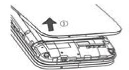
® Removing or installing the back cover.
