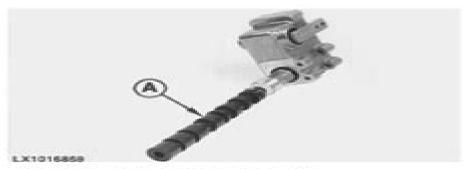
LX1016859-UN: Disengage Valve Spool Disengage the valve spool (A), and take it off.
