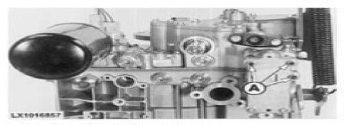
LX1016857-UN: Remove Cap Screws Take out cap screws (A).
