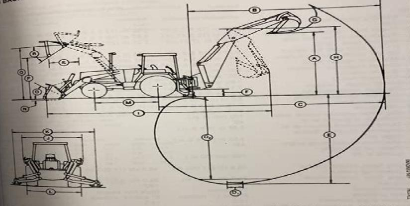
NOTE Specifications and design subject to change whost notice. Wherever applicable, specifications are in accordance with SAE Sandards. Except where otherwise noted, hese specifications are based on a standard machine with 19.5L-24 rear tires; 11L-16 front tires; 1.15 m3 (1.5 cu yd) loader bucket; 610 mm (24 in.) backhoe bucket; ROPS/FOPS; full fuel tank and 79 kg (175 lb) operator.
