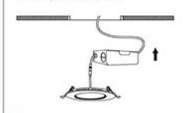
4. Squeeze the snap spring clips and push the light into the ceiling and done!
