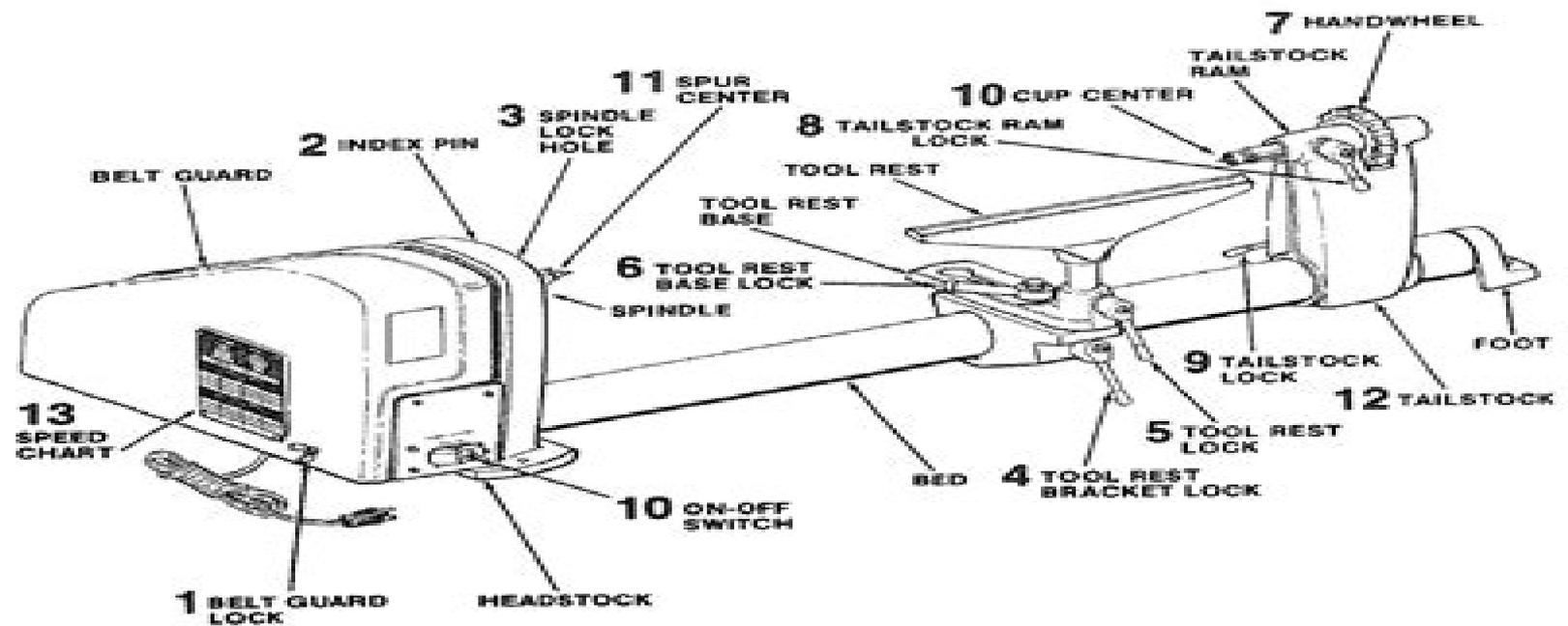
1. **BELT GUARD LOCK** . . . Locks the hinged part of the guard during operation.
