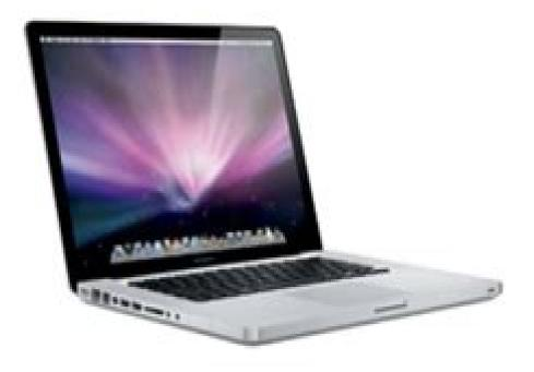
The MacBook Pro "Core i7" 2.2 15-Inch (Early 2011/Thunderbolt) features a 32 nm "Sandy Bridge" 2.2 GHz Intel "Core i7" processor (2720QM), with four independent processor "cores" on a single silicon chip, a 6 MB shared level 3 cache, 4 GB of 1333 MHz DDR3 SDRAM (PC3-10600) installed in pairs (two 2 GB modules), a 750 GB Serial ATA (5400 RPM) hard drive, an 8X DL "SuperDrive", dual graphics processors -
