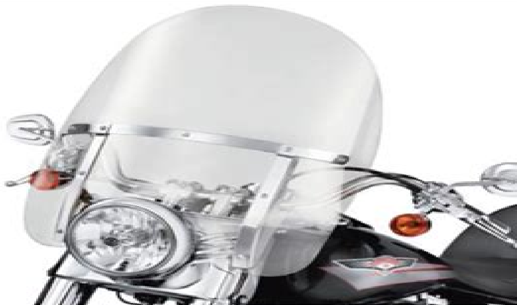
B. DETACHABLE KING-SIZE WINDSHIELD FOR FL SOFTAIL MODELS - STANDARD-HEIGHT, CLEAR
