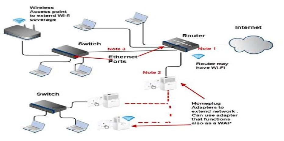
Note1: Most Home routers have several Ethernet ports and often also Wi-Fi. They also generally have a (ADSL,VDSL or Cable) modem built in but you may need an external one. If you are short of Eternet port use a switch plugged into one of the ports to extend the ports
