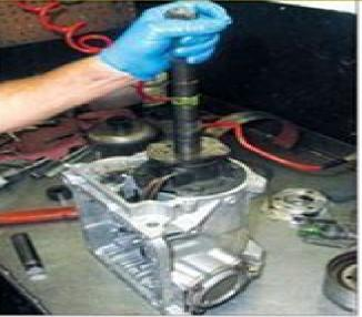
Use transmission assembly lube to *lubricate* twillshaft. seals. Install the shaft. gently working them into the governor distributor. A key to reliable assembly is being gentle. Force stubborn pieces together and you damarge critical. surfaces and powrts.
