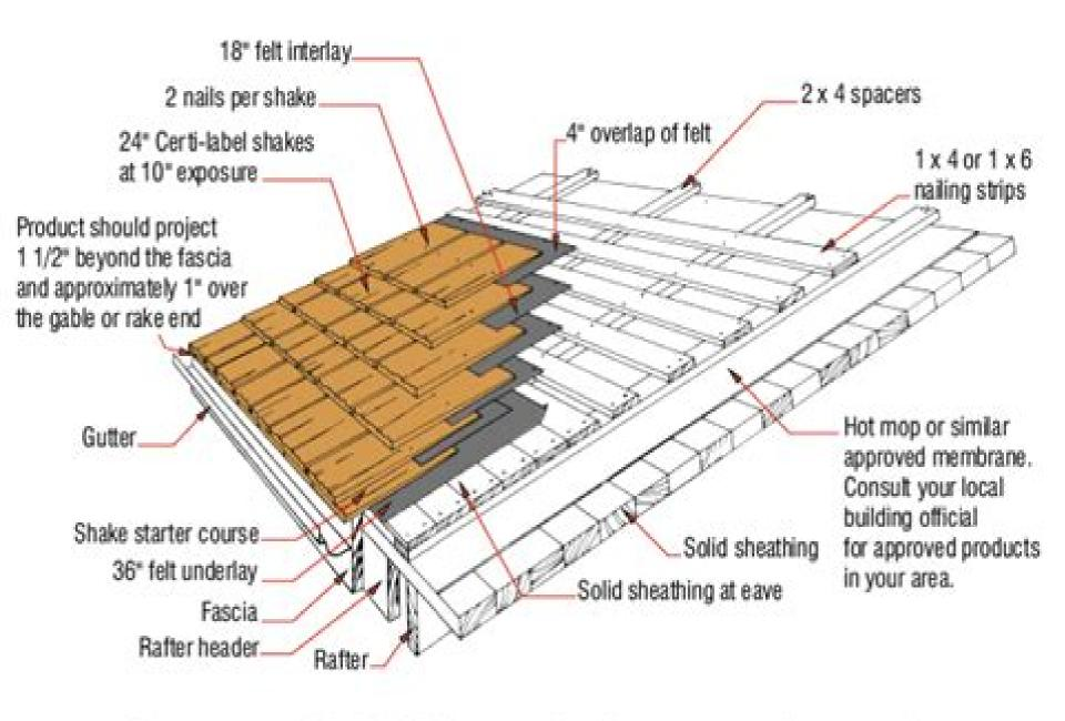
Figure 7: Certi-label Shake Application to Low Slope Roofs
