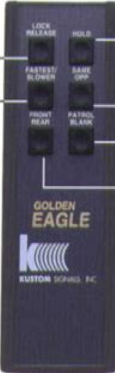
**Hold** controls the transmission of RF signal, defeating radar detectors.
