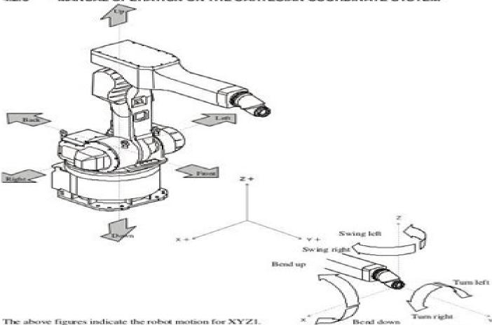
Refer to the figure for Joint coordinate system regarding the motion direction of the wrist axes ( $4^{th}$  –  $6^{th}$  axes) for XYZ2.
