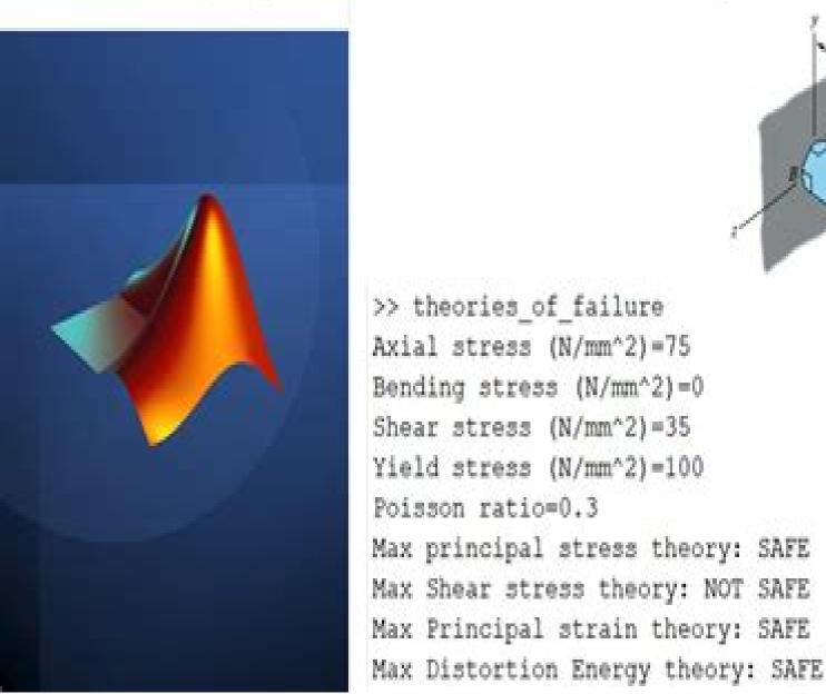
>> theories of failure Axial stress (N/mm^2)=75 Bending stress (N/mm^2)=0 Shear stress (N/mm^2)=35 Yield stress (N/mm^2)=100 Poisson ratio=0.3 Max principal stress theory: SAFE Max Shear stress theory: NOT SAFE Max Principal strain theory: SAFE
