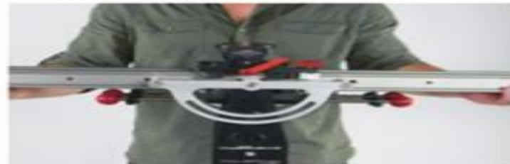
FIG 6. The "smile" quadrant of the rail system should be on the outside of the fulcrum head.
