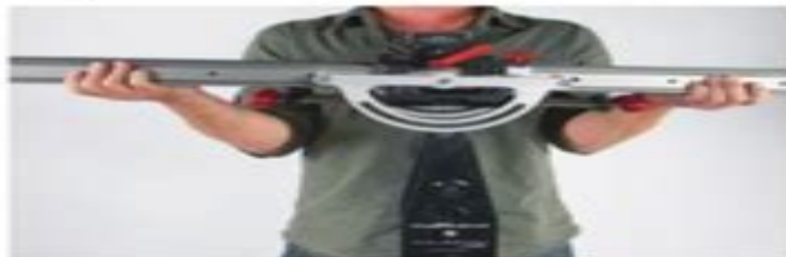
FIG 5. Insert the rail onto the top of the fulcrum with the red "kip" handle on the same side as the Matthews script.
