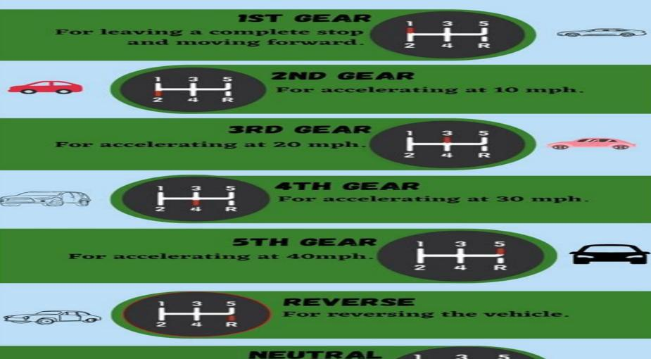
The amount of engine power available is determined by the gears. While the fifth gear has the least pulling force but the widest range of speed, the first gear has the most pulling power but the least potential for speed.
