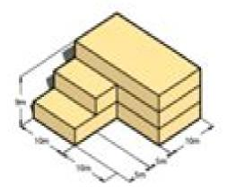
Heated Floor Area (A, J\*: 562.5 mil Envelope Area (A\_1) 1,230 m² Viplume No. 2,250 mil Heat Loss Form Factor(A\_/A\_): 2.19
