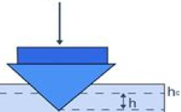
$h_0$  = Indentation depth by minor preliminary load
