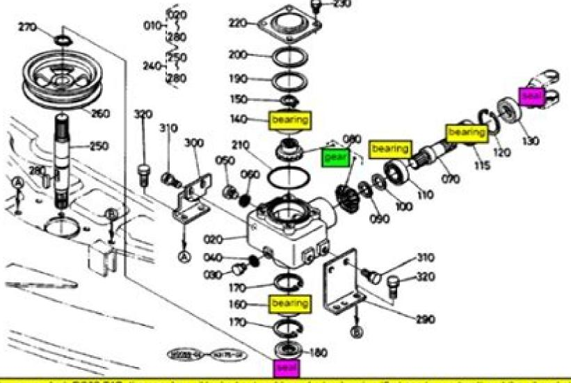
I have a Kubota mower deck RC60-71B, the gear box oil leaked out and I need a top bearing (first one to overheat) and the oil seal at the bottom of the gear box (where the oil leaked out). I have removed the top bearing no problem, but I can't tell just what to do next to remove the lower bearing(?) to get to the oil seal. Can anyone help me with a short step-by-step explanation?
